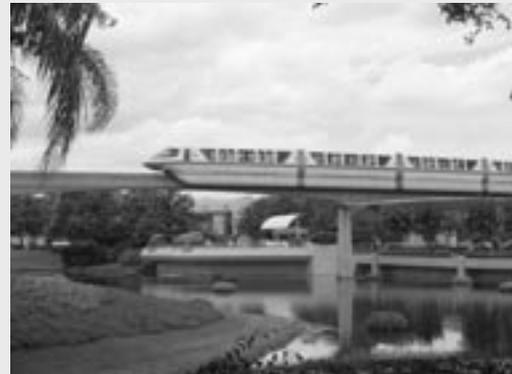
IV vehicles built by Martin Marietta. The trains are nearly identical to those that operate over 2.5-mile route at Disneyland in Anaheim, Calif. The fleet is powered by third-rail electric current alongside the track-bed, and each train is operated manually by Disney's monorail operators. Maintenance and dispatch operations are also performed by Disney staff.
