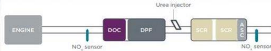
Figure 1. EPA 2010 aftertreatment system layout.
